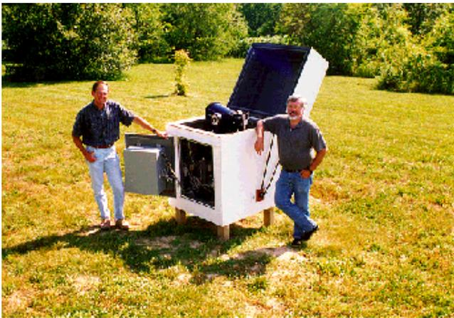
*The Hanna City Robotic Observatory robotic telescope features an 8-inch Meade LX-200 equipped with an SBIG ST-7 CCD camera and filter wheel.*
