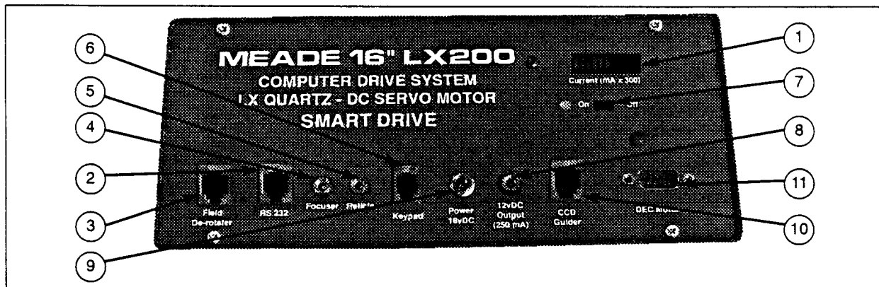
Fig. 8: 16" LX200 Power Panel. (1) Current (mA x 300) Ammeter; (2) RS-232 Connector; (3) Field De-Rotator Connector; (4) Focuser Connector; (5) Reticle Connector; (6) Keypad Connector; (7) ON/OFF Switch; (8) 12v DC Output (Fan); (9) 18v DC Power Connector; (10) CCD Connector; (11) DEC Motor Connector.
